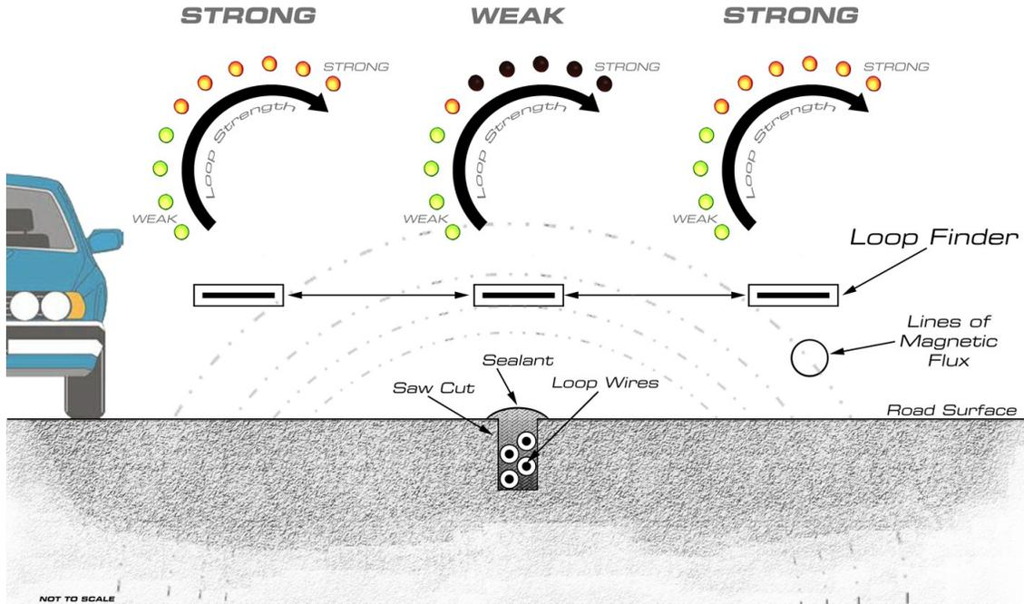
When you need to pinpoint the loop wires, reduce the sensitivity by adjusting the sensitivity switches on the face of the unit, according to the instructions on the LF-22. This allows you to hold the unit closer to the loop wires without having the loop strength reading at the maximum all the time. Continue to look for the High-Low-High pattern to locate the position of the wire, and then mark the pavement if desired.
