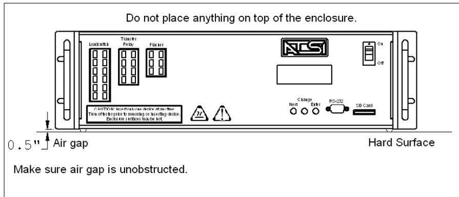
Figure 1. Tester placement.
