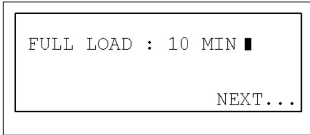
Press the CHANGE button to adjust the FULL LOAD test time in increments of 1 minute. Set this value to NONE if you do not want to run this test. Press NEXT when finished.
