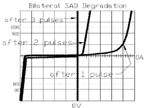
*Figure 7 P6KE220CA SAD degradation under ~300mJ pulses. Note how only the reverse-biased junction degrades and fails because of its higher power dissipation. The clamp voltage drops as the device is stressed.*
