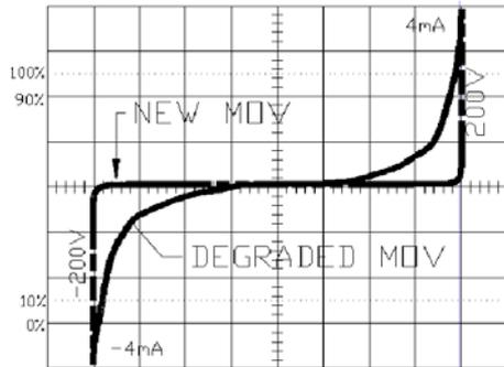
**Figure 6** Thermal runaway characteristics in a small MOV.
