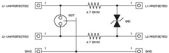
Figure 8 Data Line Suppressor
