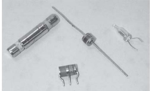
Photo 3 Gas Discharge Tubes
