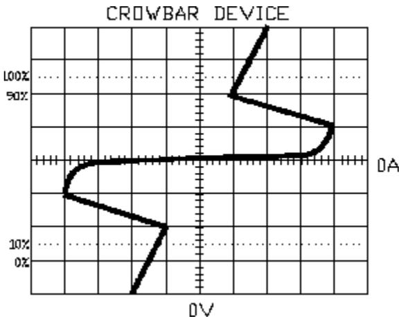
Figure 1 Crowbar Device Characteristic V-I Curve. The breakover voltage is that extreme where the curve begins to fold back. The voltage at the point at which it stops folding back is the turn-on voltage.
