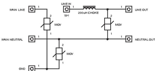
Figure 5 Line-Voltage “Hybrid” Suppressor
